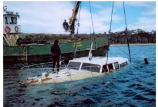
her to the waterline. There followed several hours of drama as the crane reached its maximum lift just short of the critical height to allow high pressure pumps to evacuate water quicker than it was coming in.
