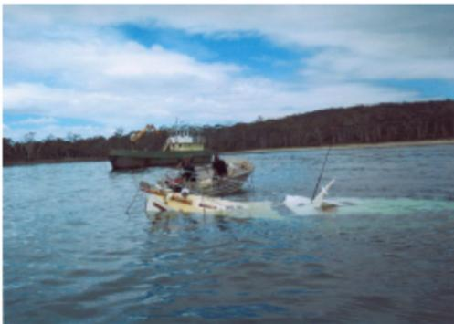
I was pretty impressed to watch guys going under with hammers, nails, tarpaulin, and scraps of plywood; they patched the damage, ran slings under 'L'Hirondelle', and then craned
