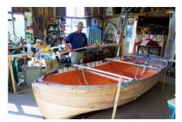
In Ned's shed the pages of the wooden boat restoration story turned. Chapter one: we'll remove the paint from the garboards and take a closer look. Hmm... not too good, looks like the keel will need replacing. At least most of the planking still looks OK. Chapter two: What did I say about the planking? Chapter three: she really would benefit from all new ribs. Chapter four, five, six... We've come this far, wouldn't a Huon pine-laid deck top the rebuild off?
